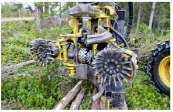
↑ In V-Tec the diagonal ribs always follow in the same direction, i.e. the left and the right roller are identical. Thanks to this design, the reverse direction also has the same grip as the forward feeding. The V-Tec range covers the commonest three- and four-roller cutting head models.
