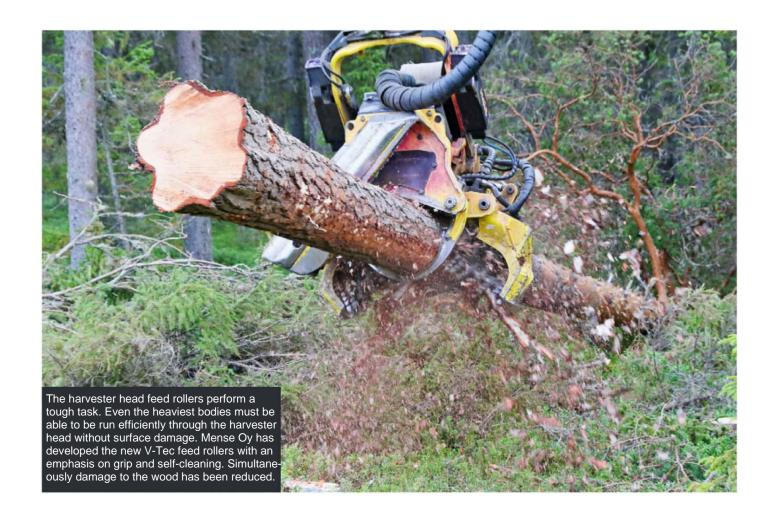
Because the teeth line is oblique, for the thickest wood bodies, the teeth form a rim as circleshaped as possible. It reduces the "digging" of the roller. Again, for thinner woods the sparseness of the ribs reduces the number of touching points of the teeth, which crushes the lure of the tree at fewer points and breakage of the tree is reduced.
