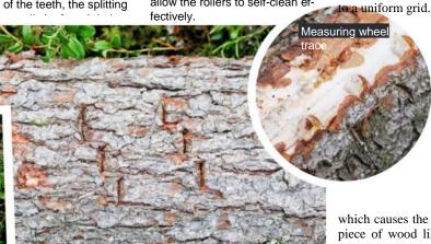
↑ ★ Because the teeth bite into the bark in-between each other, the bark does not break into pieces and is not shed so easily. The wide tooth also equalizes the surface pressure at the points where the cutter blades have removed the bark. The difference between the traditional stud teeth is significant, a curved stud leaves a sharp mark. Also the sparser teething of the measuring wheel digs into the surface of the wood.
